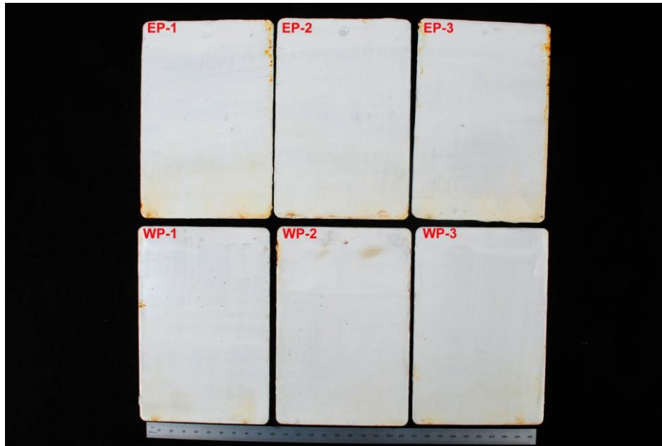
Fig. 7 The “EP and WP” Unbreached Coating (Control) panels are shown following cyclic corrosion.
